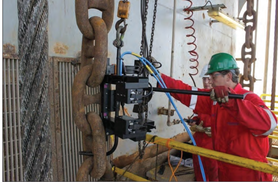
The Welaptega Chain Measurement System is used for a topside survey of mooring chains on a drill rig.
