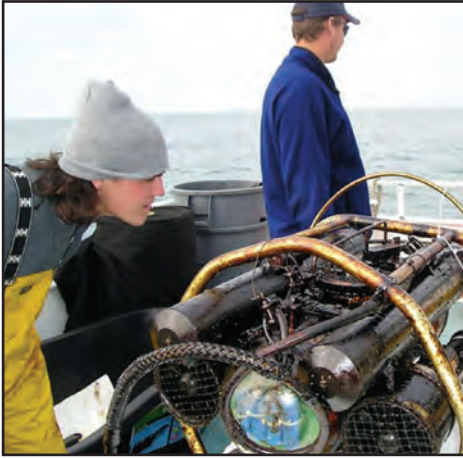
A Remotely Operated Vehicle (ROV) similar to the one above can be used to detect submerged oil. Credit: Ocean Eye/LLC and National Oceanic and Atmospheric Administration/Department of Commerce
